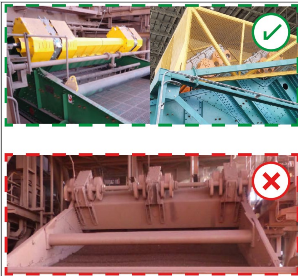
Figure 5.3-1: Exciter and drive train guarding
