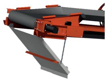
Sandvik magnetic drum separators can be retrofitted, to all Sandvik QE Range mobile scalpers to remove ferrous metal within the feed material.
